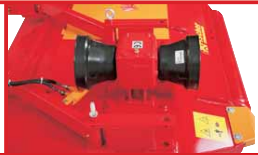
Front and rear mounting with gear drive output shaft for changing rotating direction
