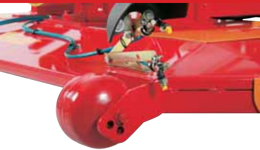
Herbicide spraying head with two own sprays
